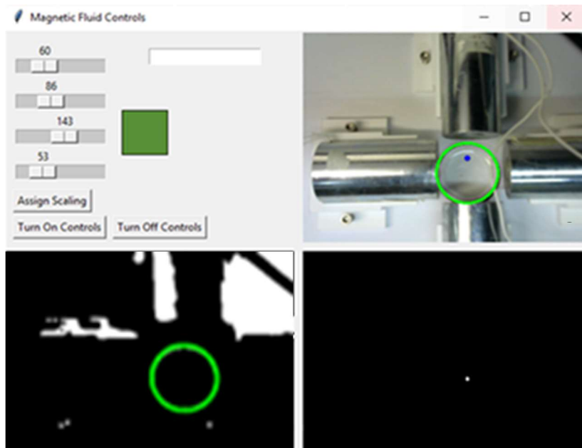
Figure 16: OpenCV GUI: A) HSC sliders and color output. B) Petri dish locator in black and white image C) Fixed Petri dish boundary in colored image D) Ferrofluid droplet locator in black and white image
